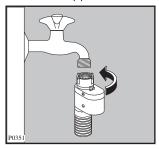
The inlet hose must not be lengthened. If it is too short and you do not wish to move the tap, you will have to purchase a new, longer hose specially designed for this type of use.
